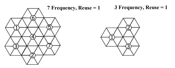
For these types of deployments, the cell reuse distance, R<sub>u</sub>, can be defined as follows:
