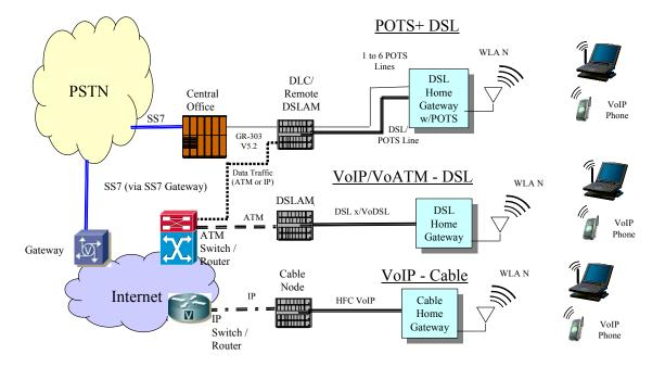
Residential/SOHO customers typically have one or more analog voice circuits which are connected directly to the PSTN through a CLASS 5 switch or through a DLC remote terminal. In many cases, subscribers are served by advanced DLC/DSLAM (DSL access multiplexer) remote terminals that provide a combination of DSL and POTS service on a single line as well as standard POTS voice circuits.
