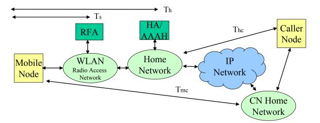
When both caller and the mobile node are in the home network (i.e. when the switching occurs within one's own voice network), the PBX function is present. In this case, the VoIP call is routed through a self-contained enterprise network and no Internet domain resources are required.
