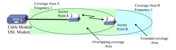
Access point B is a repeater (mesh element) to access point A, which connects to the Internet. Access point A functions as a router to access point B. Access point A must maintain a routing list for all clients in the home network while access point B only must maintain a routing list of attached clients. For example, B may be a simple bridge or a more intelligent router. Clearly, the
