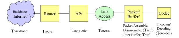
Because delay in the PSTN backbone network is beyond the control of mobile device manufacturers, the following table illustrates a residual delay budget for the backbone network (Tbackbone) using short duration G.711 and G.726 VoIP packet structures. The data for this table is taken from measurements that were performed on TI/Telogy VoIP software implementations and from worst case delays in TI's extensive wireless enterprise network.
