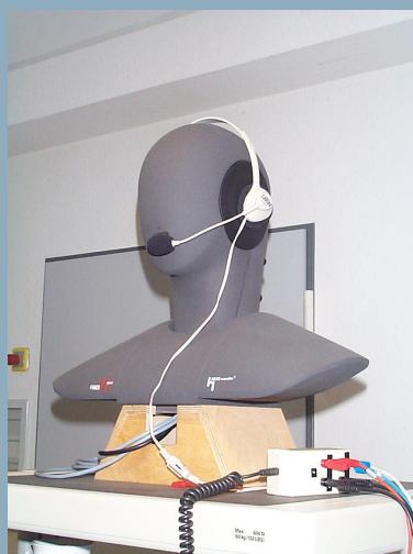
Measurement for handsets and headsets
