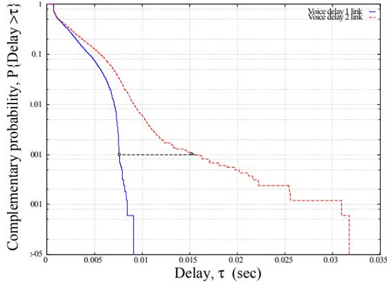
Fig 5.1 - Complementary Probability of Voice Delay:  $P\{\text{delay} > \tau\}$  - One Active Video Source
