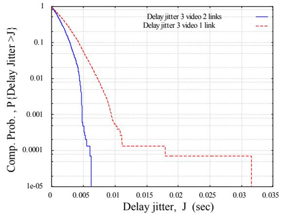
Fig 5.3 - Complementary Probability of Voice Jitter Delay:  $P\{\text{delay jitter} > \tau\}$  - Three Active Video Source
