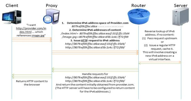
The architecture diagram of our IPv6 content addressing system. In our system, the regular browser makes a HTTP request through a proxy, which translates HTTP requests to an IPv6 content addressing system. The request is sent out over the network, until a router on path that has the content responds to the request. The proxy then translates the retrieved content back into a HTTP response to the user's browser.
