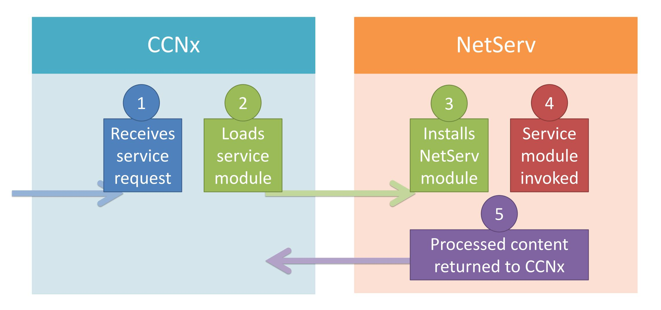
The architecture for our CCNx dynamic service scalability implementation. When CCNx receives a content request that it interprets as a service, it loads the service module (over CCNx), processes the content using the module in NetServ, and then publishes it in CCNx space.
