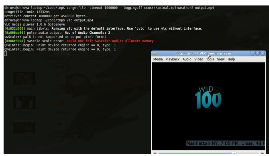
A processed content is obtained through CCNx and played in VLC media player. There is a small watermark with weather information at the bottom right of the video, showing that this is processed video obtained from CCNx.
