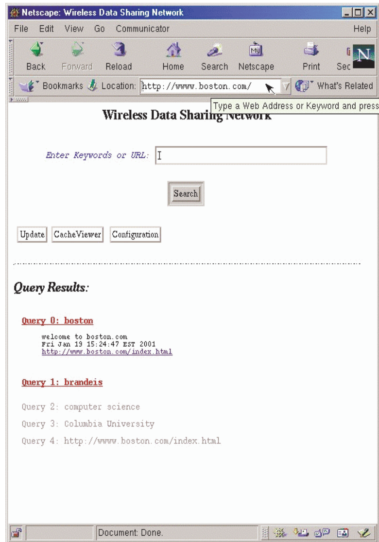
Figure 2.8: 7DS main GUI. In the upper part of the GUI, the user can enter a URL or form a keyword-based query or view the cache manager or configuration. Query results are in the lower part. In this example, queries 2, 3, and 4 are pending, whereas there are responses for query 0 and for query 1. The query 0 is “expanded”, i.e., showing the report.
