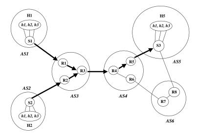
Figure 3: Example of a sink tree rooted at  $S_3$
