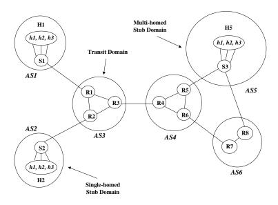
Figure 2: Example of Internet domains. There are two types of stub domains: *single-homed* stub domains connect to the backbone at a single point, *multi-homed* stub domains at several points.
