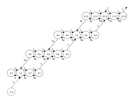
Figure 9: State transition diagram for  ${\cal Q}=3$
