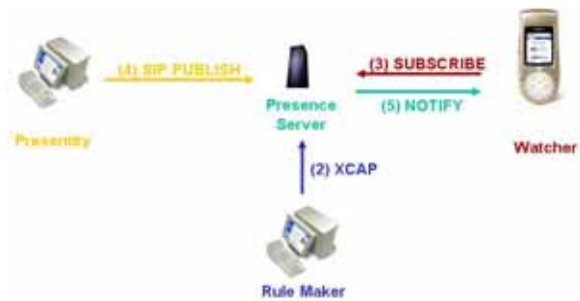
Fig. 2. Example of a location-based Instant Messaging Application
