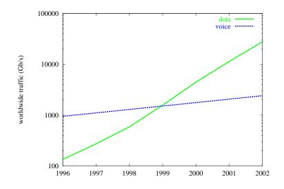
voice traffic  $\ll$  data traffic  $\rightarrow$  design network based on "data" traffic  $\rightarrow$  IP as common transport
