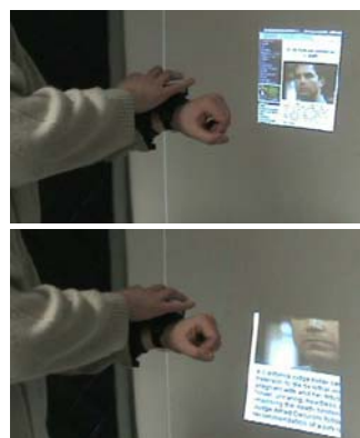
Figure 1. Use of simulated wrist-worn projection system to explore interaction possibilities: Panning, zooming, and interaction with content is possible with the use of orientation- and position-tracking technologies and virtual widgets implemented on the wrist-worn system's touch-sensitive surface.
