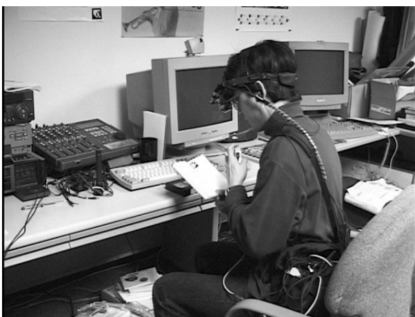
Figure 5: Wearable system is used to attach a voice note to the physical object
