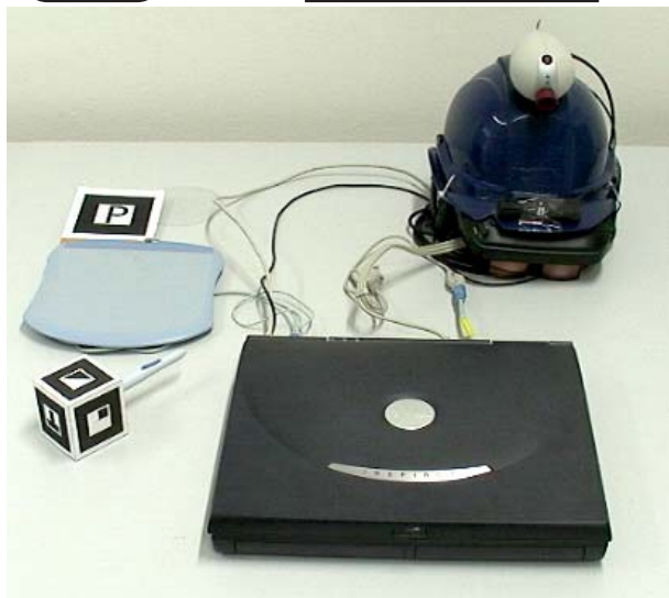
Figure 4. All components of the mobile setup are commercial items: (top) hardware design diagram, (bottom) picture of the components
