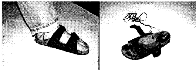
Figure 5: The shoe provides a convenient location for sensor placement. Here, a skin conductivity sensor is placed in the arch of the shoe and a pressure sensitive resistor is placed on the heel. Sensors look unobtrusive when worn. (Photograph courtesy of Fernando Padilla)
