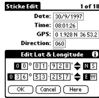
Figure 2. Manually editing a location field of a stick-e note in the StickePad. The 'Here' button retrieves the current GPS value.
