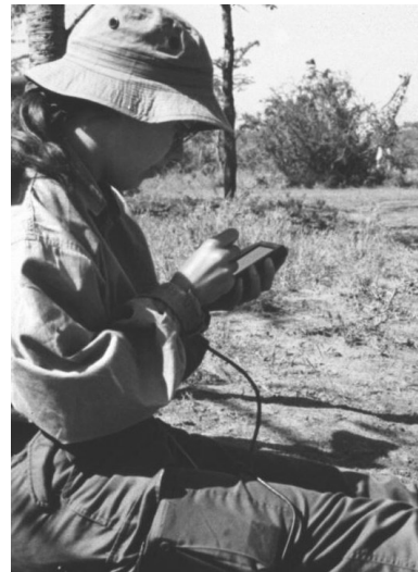
Figure 1. The Ecologist records an observation of a giraffe (see top right of photograph) using the 3Com PalmPilot linked to GPS-enabled trousers.
