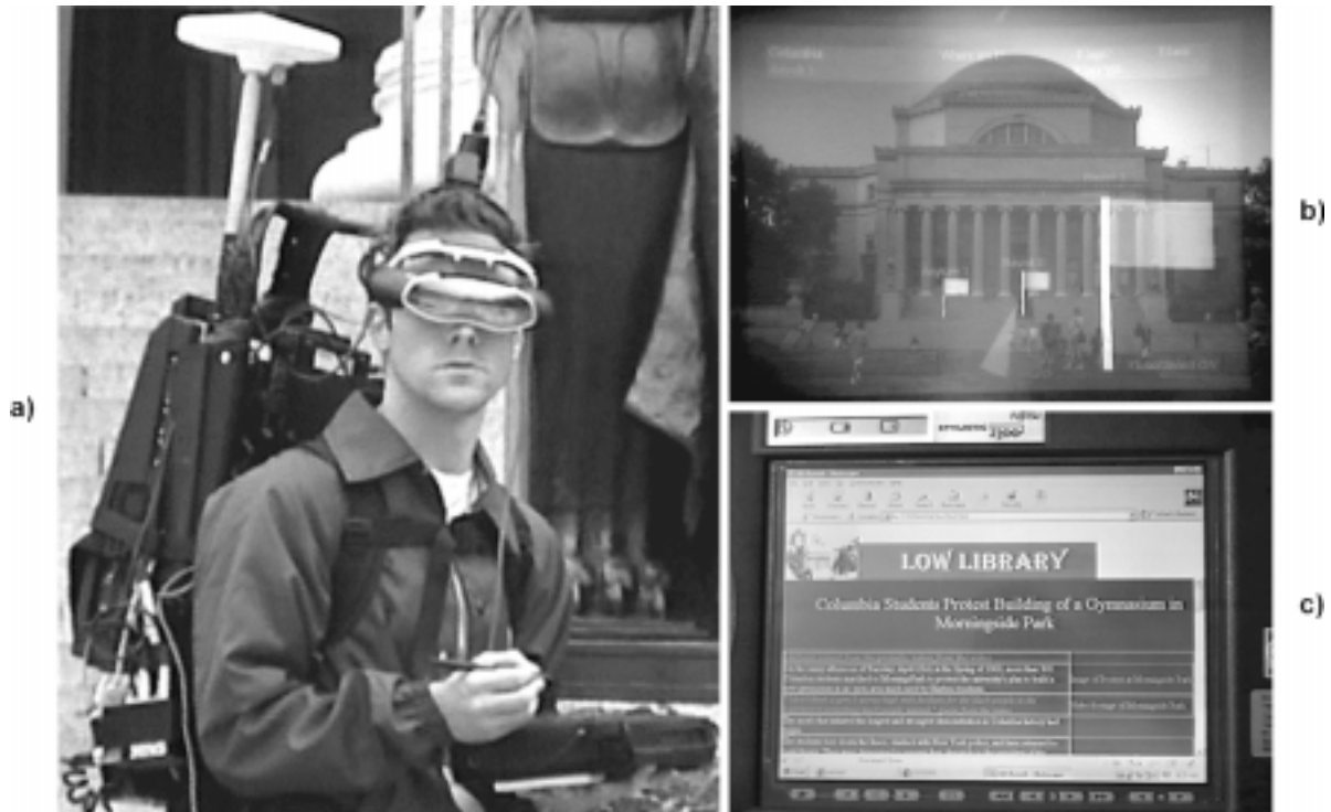
Figure 1. Situated documentaries. a) Our backpack-based testbed, with tracked see-through head-worn display and pen-based hand-held computer. b) An image photographed by a video camera that wears our testbed's see-through head-worn display. The labels and virtual flags are part of the user interface, described in Section 3. c) Related information displayed on our hand-held computer.
