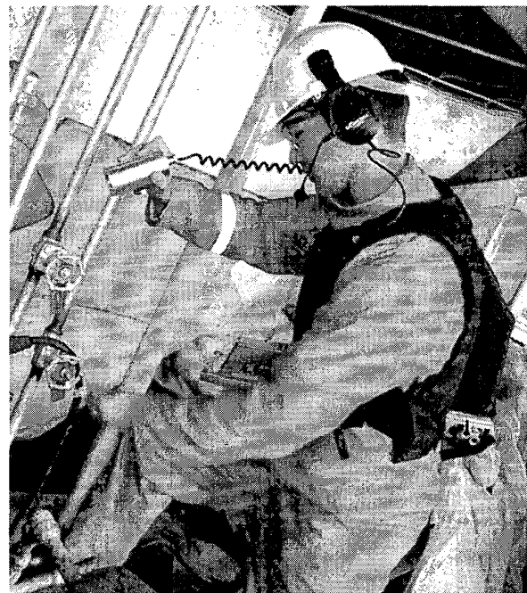
Figure 5: Using EX-certified wearable computer in area where there is a danger of explosion.
