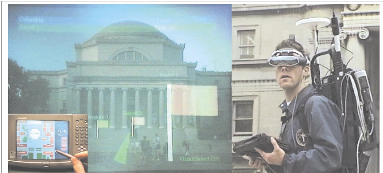
■ Figure 3. The “Touring Machine” mobile augmented reality system presents information using a tracked see-through head-worn display and a stylus-based handheld display. A handheld map of the campus is shown at left, an annotated real-world view through the see-through head-worn display at center, and the current backpack testbed at right.
