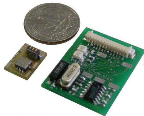
Figure 3. Image of the accelerometer components compared to a coin.
