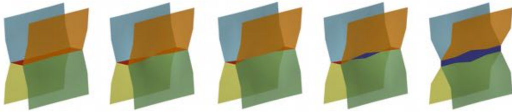
Figure 6.3: A 3D T1 process begins when a short edge between distinct triple-junction curves collapses to become a vertex incident on four materials. Adjacent edges on the original interface (red) also collapse yielding a quadruple-junction curve. Then, one vertex on the curve separates perpendicularly to create a new interface (dark blue). Nearby vertices follow suit to complete the process.
