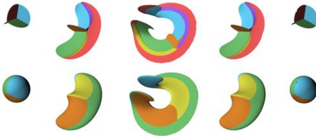
Figure 10.1: Multimaterial Enright test: A sphere divided into four material regions is advected through the “Enright test” velocity field. The distinct regions are well-preserved despite the extreme stretching. Top: Interior interfaces. Bottom: Exterior interfaces.
