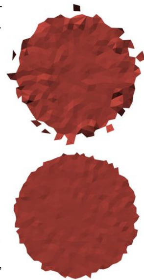
Figure 10.5: Mean curvature flow: A collection of 2000 random Voronoi cells undergoes many T1 and T2 topology changes.
