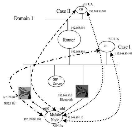
Fig. 1. Heterogeneous SIP in a LAN: Scenario 1
