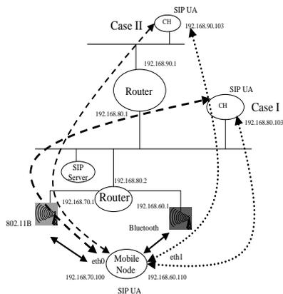
Fig. 2. Heterogeneous SIP in a LAN: Scenario 2
