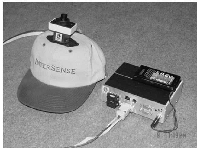
Figure 5: Photograph of prototype self-tracking system.
