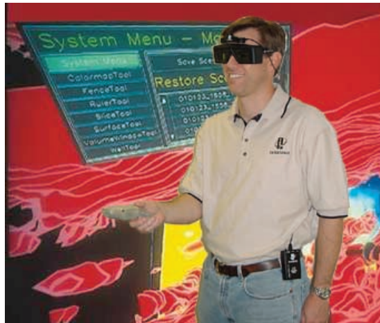
12 InterSense IS-900 wireless tracker option, including a belt-worn battery/radio module for the head tracker. For the head wand, the battery and radio are built into the handle.
