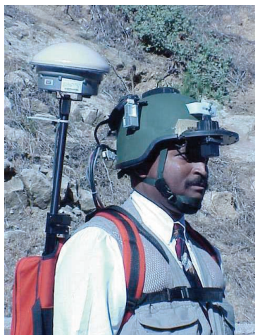
10 HRL Laboratories prototype person-portable mobile augmented reality system with GPS, inertial, and magnetic sensors.
