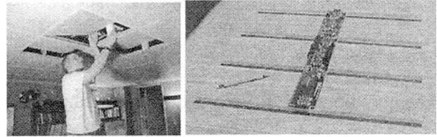
Figure 3. Left: Bishop lifts some Ceiling panels. Right: an individual Ceiling panel module showing the main PC board with four LED strips (eight LEDs per strip).
