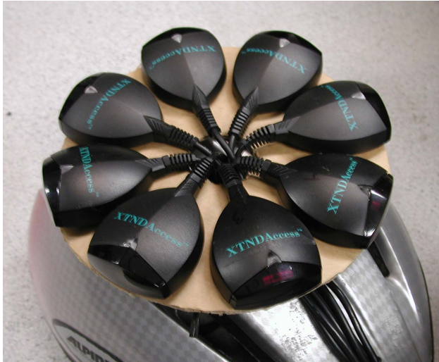
Figure 2. Dongle array on test helmet
