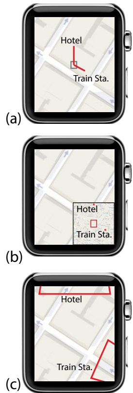
Figure 4: Where am I? Localization on a smartwatch form factor using (a) P-Compass, (b) Overview+Detail, and (c) Wedge. (© 2016 CGUI Lab, Columbia University.)
