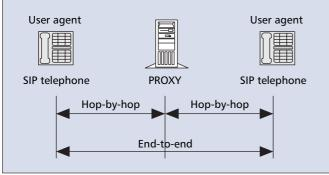
**Figure 4.** *SIP security mechanisms.*
