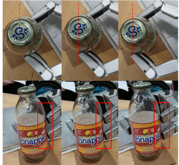
Fig. 1. Grasp adjustment using tactile experience, an example that illustrates the progression of hand adjustment. Initially, the grasp (the left column) barely touches one side of the bottle and the finger surface does not align well of the surface of the bottle. After two hand adjustments, the final grasp (the right column) has opposing contacts and the finger surface aligns with the surface of the bottle.
