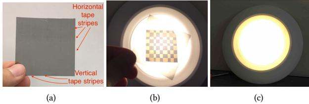
**Figure 1:** A polarizer film with horizontal and vertical transparent tape stripes arranged in a grid (a). Attaching this film to a light cover and viewing it through another polarizer, we observe colored grids (b). This pattern, however, is imperceptible without a polarizer (c).
