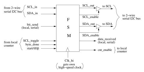
Inputs *SCL\_in* and *SDA\_in* are the bi-directional I2C bus wires; they come directly from the global I2C bus. Any changes on the I2C bus are always observable by the master controller on these 2 input wires at all times.
