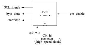
Generating the System Clock, SCL\_out: Basic Operation. The interaction of two signals, cnt\_enable and SCL\_toggle are used by the master control to generate the pulses of the system clock, SCL. Basically, the
