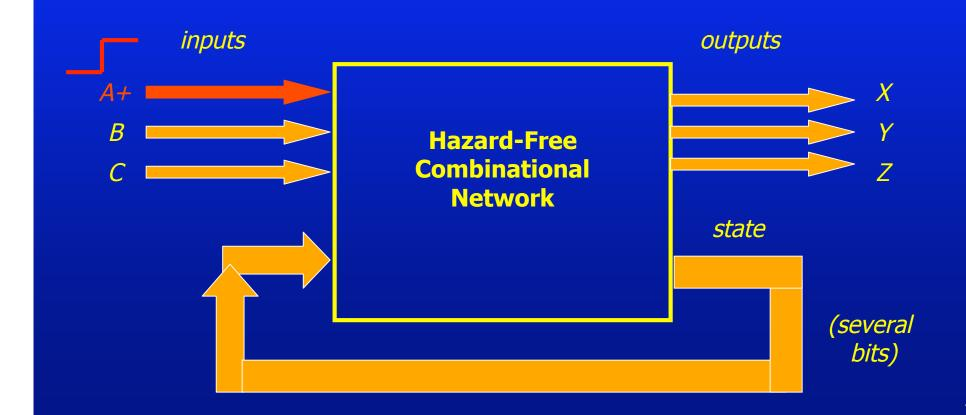
Burst-Mode Behavior: inputs in a user-specified 'input burst' arrive, in any order
