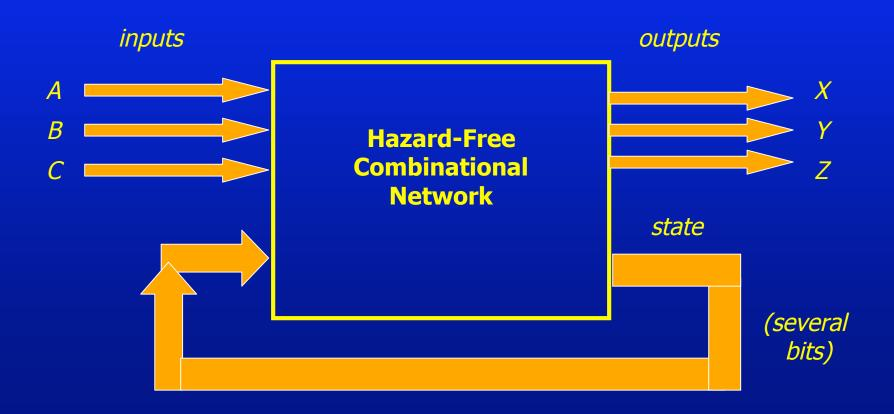
Burst-Mode Behavior: inputs in a user-specified *input* burst' arrive, in any order (glitch-free)
