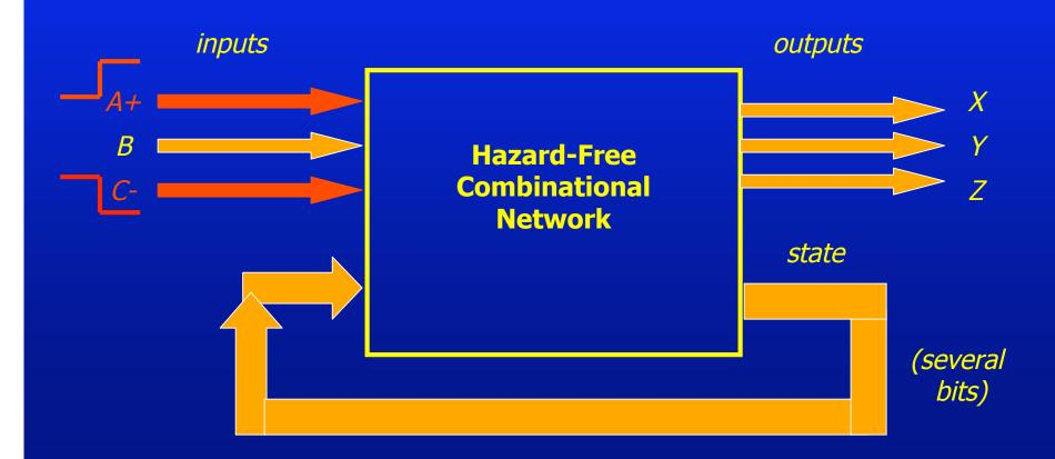
Burst-Mode Behavior: once 'input burst' is complete, machine generates a (glitch-free) 'output burst' ...
