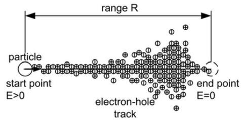
Fig. 1. Electron-hole track created by charged particle.
