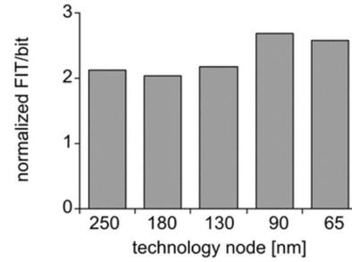
Fig. 29. Scaling of neutron SER in SRAM.
