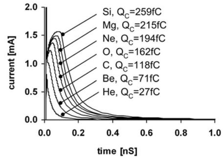
Fig. 8. Collected charge for various secondary particles with track length of 5 $\mu$ m.
