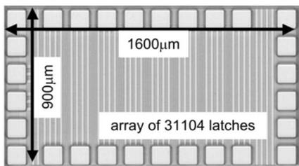
Fig. 24. Testchip photograph.
