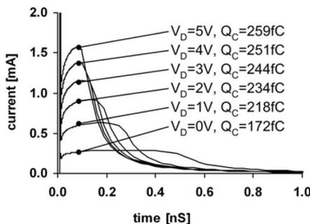
Fig. 7. Variation of collected charge and current waveform shapes with applied drain voltage.
