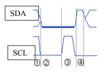
The slave that is going to send an ACK holds the SDA line low immediately after reception of the 8<sup>th</sup> bit transmitted, or, in case of an address byte, immediately after evaluation of its address. In practical applications this will not be noticeable.
