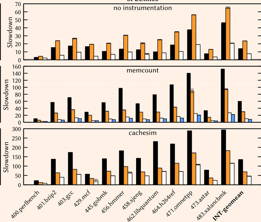
Qelt faster than the state-of-the-art, even for heavy instrumentation (cachesim)
