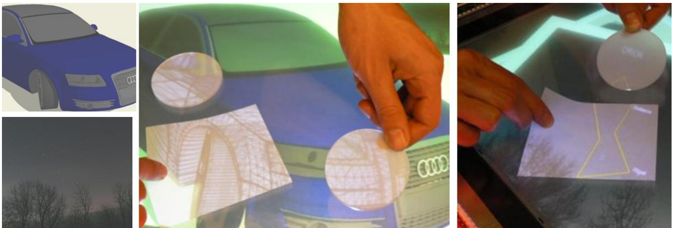
Figure 4: Creating tangible layering effects is extremely simple with SecondLight. A translucent sheet of diffuse film is placed above an image of a car to reveal its inner workings (middle) or above the night sky to reveal the constellations (right). Plain images are shown on left. Circular acrylic discs with diffuse topsides can be used to create a magic lens effect. Note how the magic lens image is maintained even if the disc is lifted well away from the surface.
