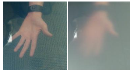
Figure 2: A switchable screen, in clear state (left) and diffuse state (right). Note: the hand is very close to the underside of the surface.
