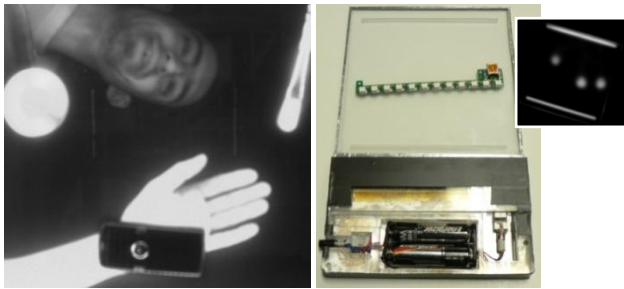
Figure 13 Left: an example image captured in the PSCT clear state. Here we obtain a far greater depth of field than other rear projected surfaces. A mobile phone, magic lens and paint brush are touching the surface, but further away we can image the user’s entire arm and even face through the surface. Right: a simple mobile surface that uses FTIR to generate a signal for tracking to enable perspective correction. The LED strip which is mounted on the side is shown resting on the center of the device. This device also generates a multi-touch signal, which, along with the edge markers, can be imaged by the SecondLight IR camera. The output captured by the camera is shown inset, here three fingers are touching the surface and the two strips highlight the edges of the display surface.
