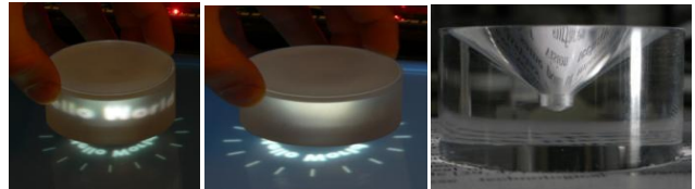
Figure 6: The ability to shine light through the display, gives rise to other novel tangible object designs. In this example, we demonstrate an object that uses internal prisms to project the incoming light onto its sides. The prism inside the object is shown right. The effect of the prism on the projection is shown left. This middle image shows the screen in a non-switching diffuse state – illustrating the behavior of a typical projection screen.
