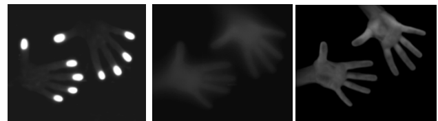
Figure 12: two hands imaged using FTIR (left) and diffuse illumination with the PSCT in diffuse (middle) and clear states (right)
