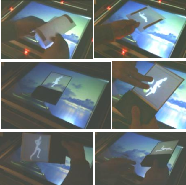
Figure 5: Mobile projection surfaces with passive and active markers being held at different orientations above the surface. The markers define the location of the object, which is tracked using the camera imaging through the surface. This allows correction of the through projection enabling it to be distortion-free and appear centered on the mobile surface. Top: a flexible sheet with passive retro-reflective marker strips. Middle: an actively tracked surface with its own battery-powered IR light source which also allows multi-touch input on the mobile surface to be sensed through the SecondLight surface (middle right). Bottom: the projected image can be corrected for distortion as it is moved and tilted, thereby supporting quick and natural reorientation into more conformable viewing positions. For example, tilted vertically towards the user or oriented towards another user for viewing.
