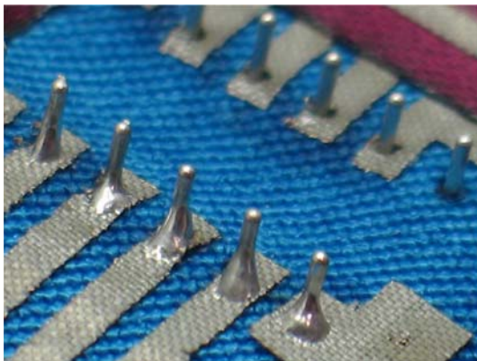
Fig. 2 Solder joints on a fabric PCB
