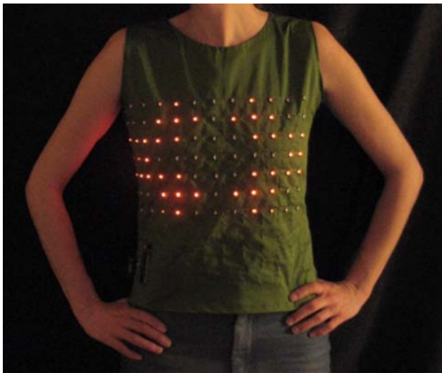
Fig. 8 A wearable LED display matrix: a shirt embellished with LED sequins
