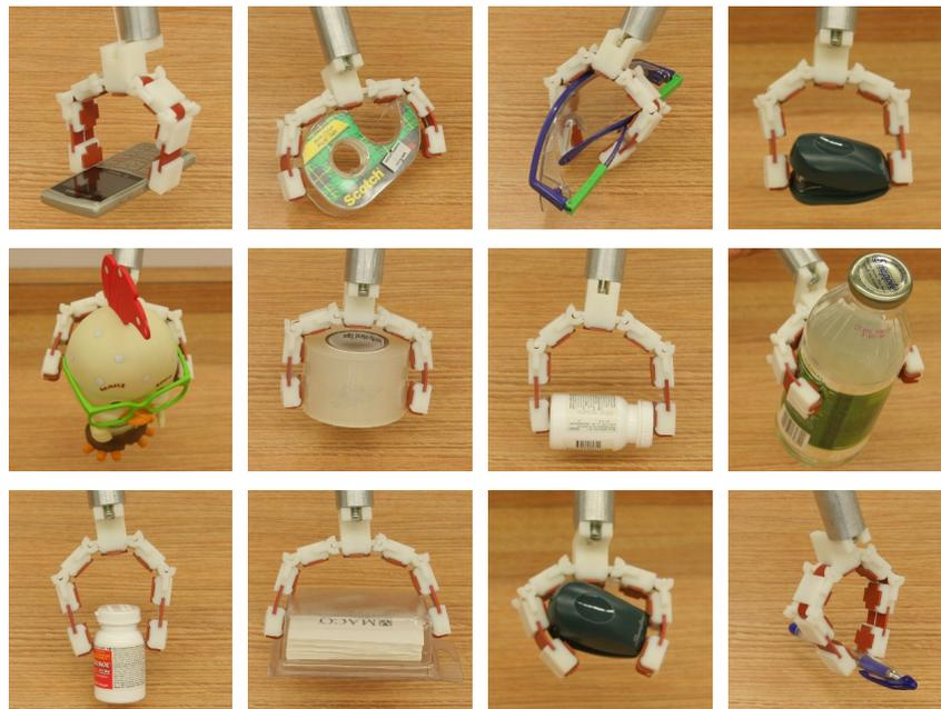
Figure 6.10: Examples of grasps successfully executed using the prototype gripper.
