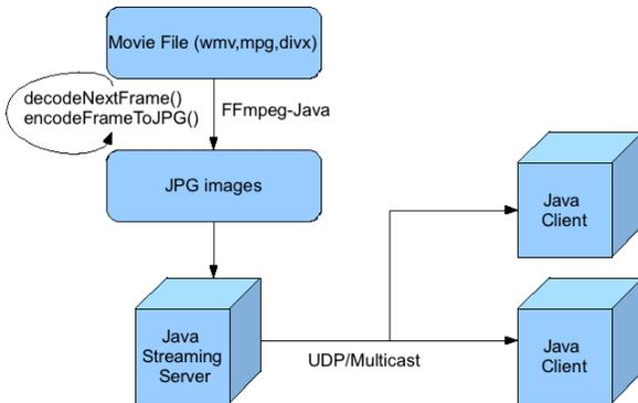
Figure 10: Transcoding a movie into JPEGs
