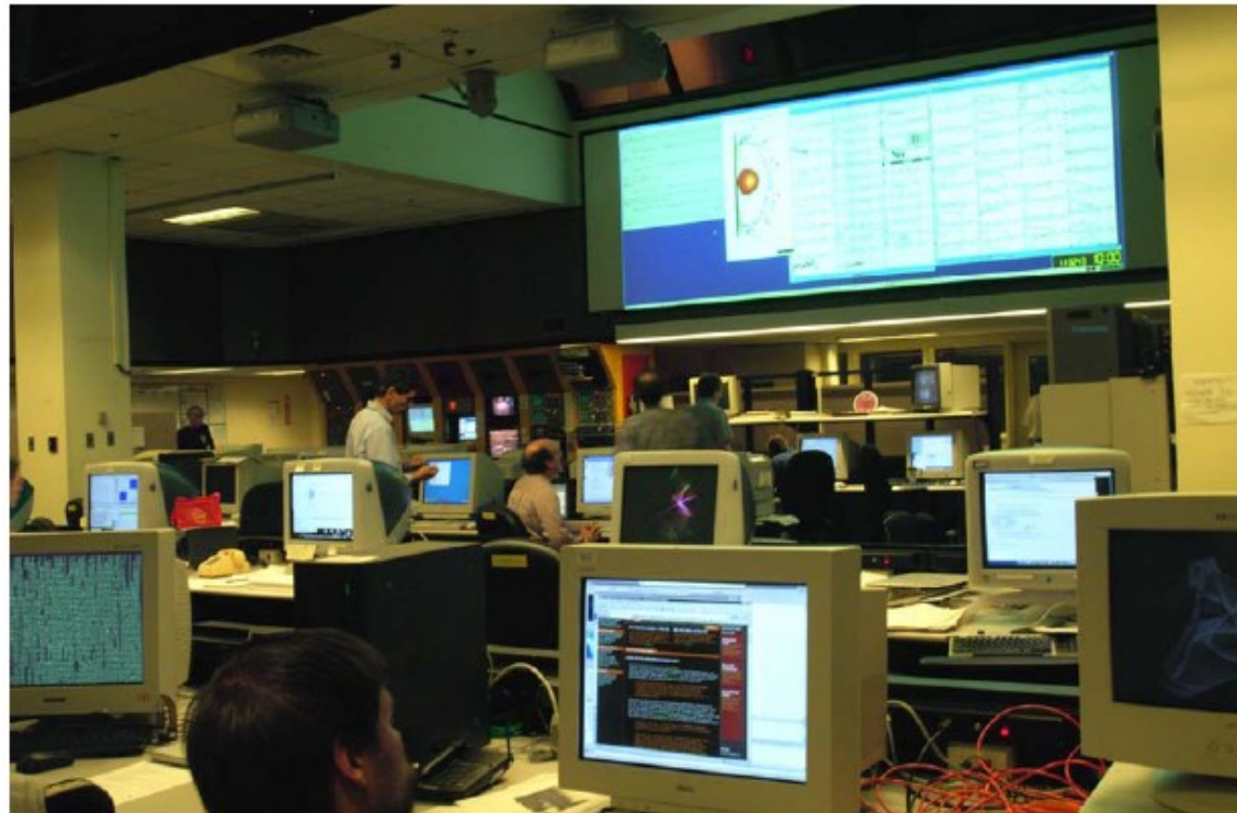
Figure 3: Shared Display Wall deployed in the NSTX control room of Princeton Plasma Physics Lab. Tens of data plots from multiple scientists are shown on the shared display. A camera shot of the plasma and also a log are also shown on the left.
