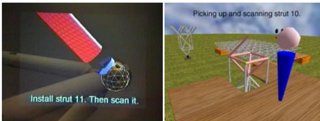
(a) What the worker sees through their head-worn display during the installation of strut 11 (see Figure 2-8).
