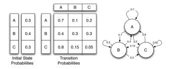
**Figure 1**. Initial state probabilities, transition matrix and graphical representation of a simple first-order three-state Markov chain.
