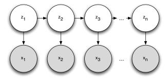
**Figure 4.** Graphical model representation of a first-order HMM.  $z_{1...n}$  are the underlying states associated with the n observations  $x_{1...n}$ . The  $x_i$ 's are shaded to show that they are observed directly. Each observation  $x_i$  is drawn from the distribution associated with state  $z_i$ , and therefore depends on  $z_i$ . Each state  $z_i$  depends on the previous state  $z_{i-1}$ .
