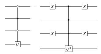
The first circuit applies U if the first three qubits are  $|0\rangle |1\rangle |0\rangle$  (the first and third dots should be empty).
