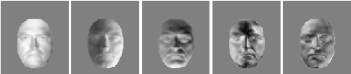
Figure 4: The eigenvectors calculated from the sparse set for the human face. Note that the images were only lit from the right so the eigenvectors are not perfectly symmetric. Observe also that the first three eigenvectors appear to be images of the face illuminated from three orthogonal lighting conditions in agreement with the orthogonal lighting conjecture.
