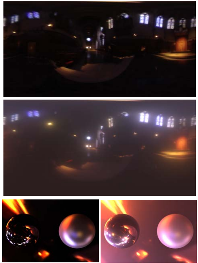
Figure 15: [Top] Grace cathedral environment map with no scattering. [Middle] The environment map is convolved with the airlight single scattering PSF to create a foggy/misty appearance. Notice the glows around the light sources, the blurring of the sources and the brightening of dark areas. [Bottom] A scene illuminated by the environment map without scattering (left) and with scattering (right). Notice the spreading of the highlights and brightening of the spheres due to scattering.
