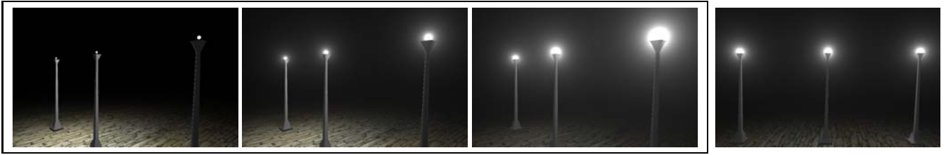
Figure 8: The images show glows around three identical point light sources (street lamps) at different distances from the viewer. From left to right, we show three different values of the scattering coefficient \beta ( \beta = 0, 0.01, 0.04 ). Larger values of \beta correspond to larger optical thicknesses T_{sv} . We clearly see the effect of greater glows for larger \beta . Also, the radiance from farther light sources is attenuated more in each individual image, resulting in smaller glows for the farther lights. In the fourth (rightmost) image, we show a different view with \beta = 0.04 , where all the light sources are approximately equidistant, with the result that they have similar glows. (The shading on the surfaces is computed using the surface radiance model in section 4.)
