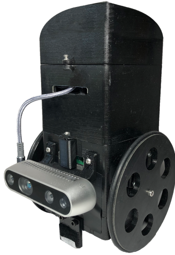
Fig. S2. Physical Robot Demonstration. Our physical robots are two wheeled robots with a first-person RGB-D camera.
