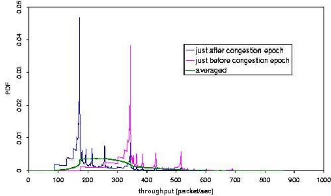
FIGURE 15. Stationary pdf of the rate of one flow with slow start;  $C=270$  Pkts/s.,  $p=.8$ ,  $1/\mu=2000$  Pkts,  $1/\beta=2$  s.
