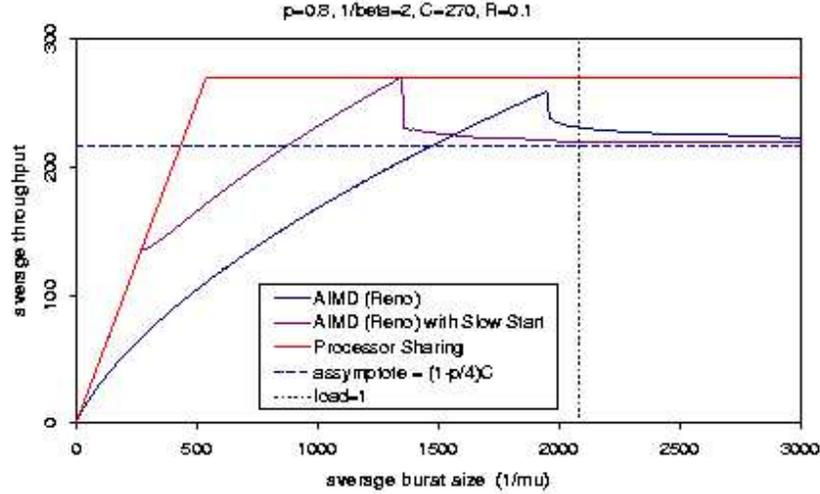
FIGURE 16. The average rate as predicted by the PS and the AIMD models.
