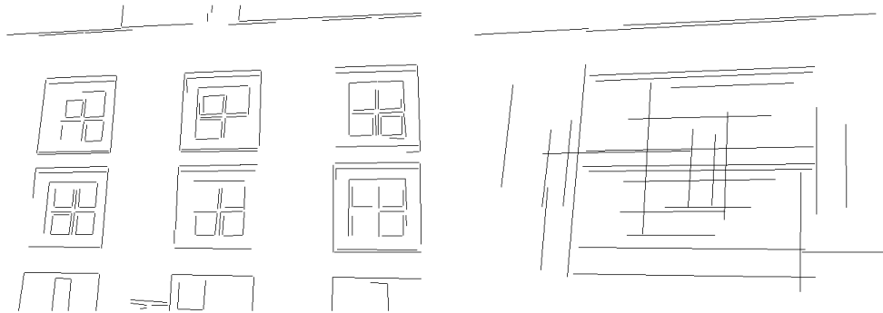
Figure 5.5: Preprocessing of the 2-D line segments: the extracted edge lines (left) and the result after merging the collinear subsets and removing the short ones (right).
