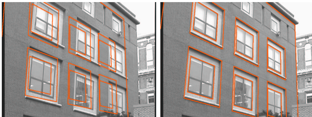
Figure 6.9: Visual localization test: Location 5
