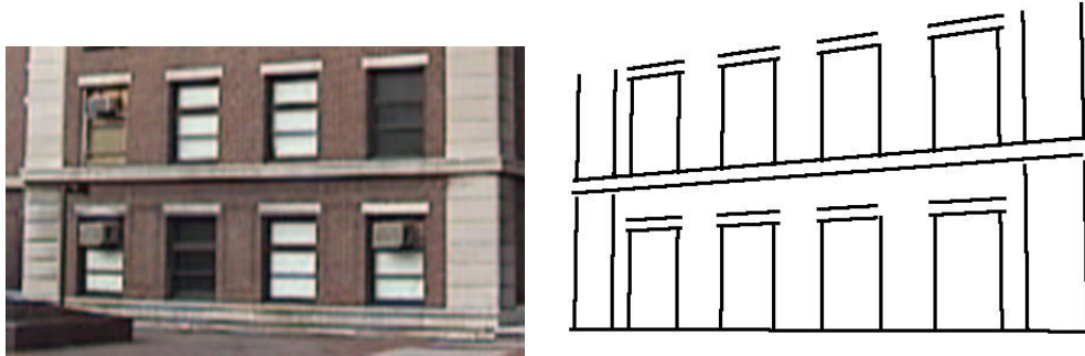
Figure 5.1: A sample model (right) of a building facade (left)
