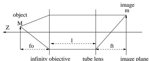
**Figure 2:** Simplified ray diagram for an infinitely focused optical microscope
