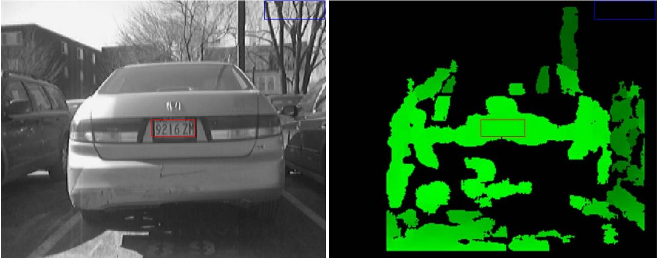
Figure 5-2: Stereo imagery rejects false alarm from text detector
