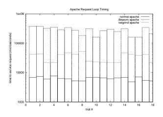
Figure 4: Timing of main request processing loop. The y axis is on a log scale and shows the overhead of running the whole primary request handling mechanism inside the emulator. Each trial represents a user thread issuing an HTTP GET request.
