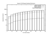
Figure 2: Performance of various levels of emulation. While full emulation is fairly invasive in terms of performance, selective emulation of input handling routines appears quite sustainable.
