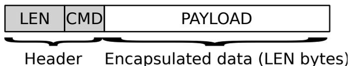
**Figure A.4:** The cascading rescue points protocol encapsulates user data using a small header prepended to every data write made by the user.
